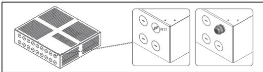
3. Break the selected parts of the perforation. In accordance with the required cables to break the selected parts of the perforation to use your cable connection.
